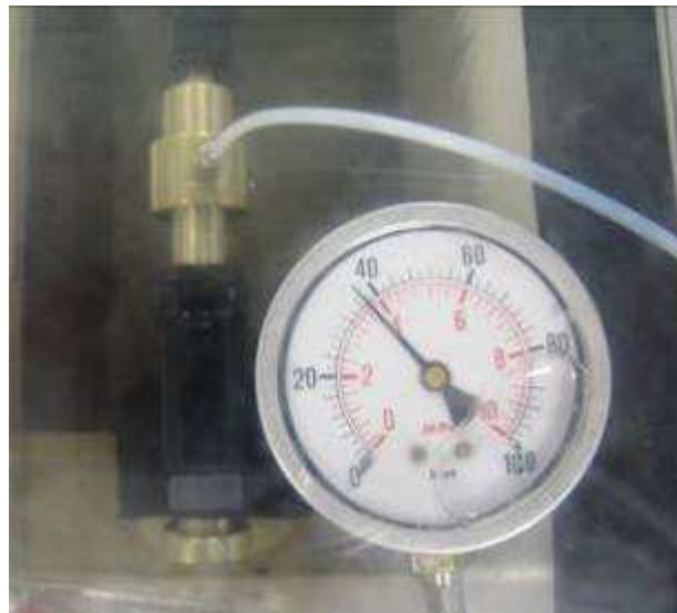
Picture n° 2 Quick connectors burst pressure - Testing modalities -
