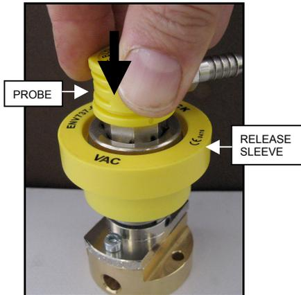
3. Insert the probe into the socket with enough force to oppose the upstream pressure, until the release sleeve of the socket clicks into place;
